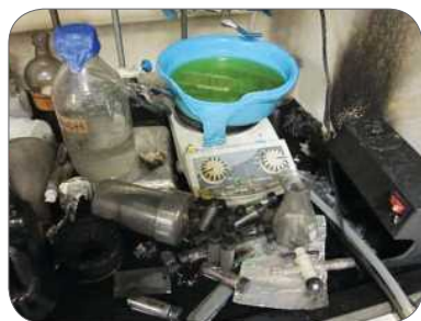
Figure 3: Aftermath of a flash fire in a fume cupboard.
