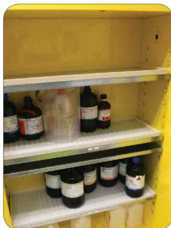
Figure 11: Storage cabinet for flammable chemicals with cabinet doors closed (top) and open (below).
