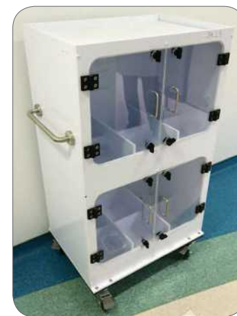
Figure 17: A chemical utility cart with 12 separate compartments for moving chemical containers.
